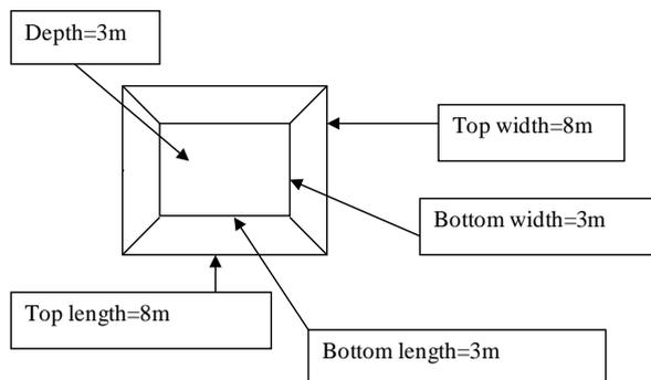
**Figure 5.** RWH pond geometry.
